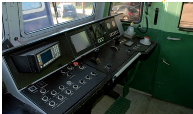
Upravený riadiaci pult na stanovišti rušňovodiča. Nové rozloženie ovládacích prvkov prijala obsluha pozitívne. / A revamped control panel in the engine driver's cabin. The new controls layout is viewed by the drivers positively.
